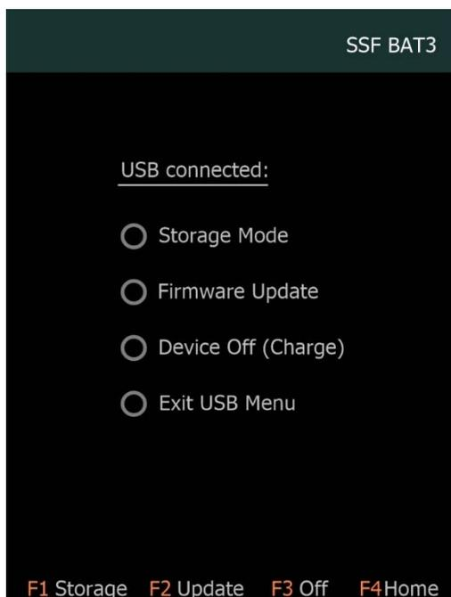
When switching on the SSF BAT3 with plugged in USB data cable the USB Menu starts automatically. The menu can also be activated via the About menu.
